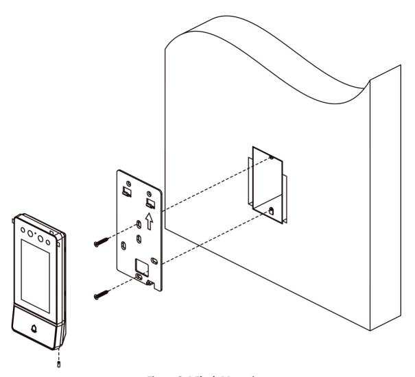
Figure 3-4 Flush Mounting
