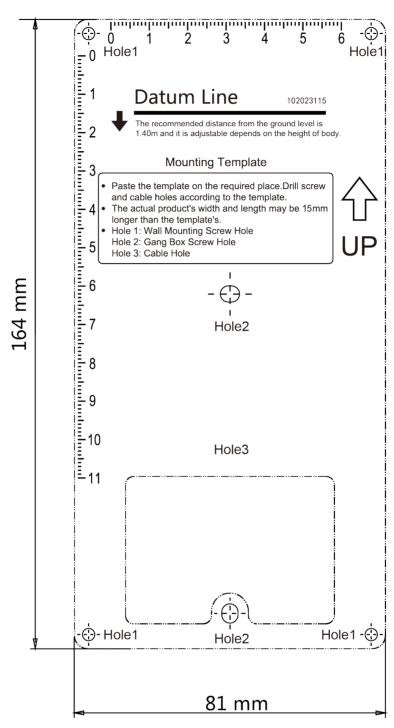
**Figure 3-2 Mounting Template**
